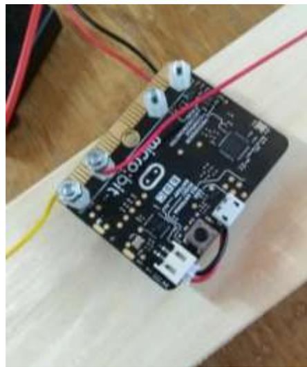
Connect trigger wires to **Pin0** and **Pin1**. Both circuits return to **GND**.
