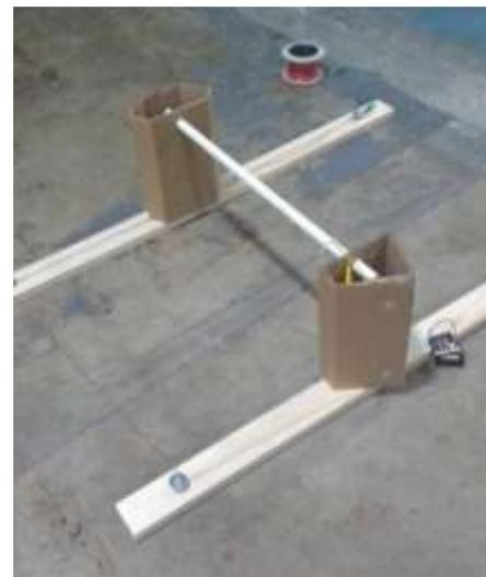
Set the gate at least 50cm wide to ensure cars do not hit it. In this team's design, a plastic tube carries the wires returning to GND over the track and tether.
