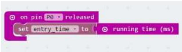
Drag out an **on pin \_\_\_ released** block from the **Input > More** section. Set it to button P0. From the **Variables** section drag out a **set \_\_\_ to** block and attach **running time (ms)** from the **Input > More** section to it.
