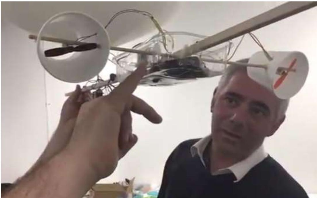
*A plastic container on a balsa spar contains the electronics and a servo that can tilt the two independently controlled motors in their foam cup nacelles 180 degrees.*
