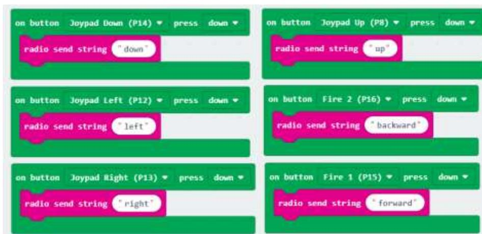
*Example of multiple commands used on a transmitter*
