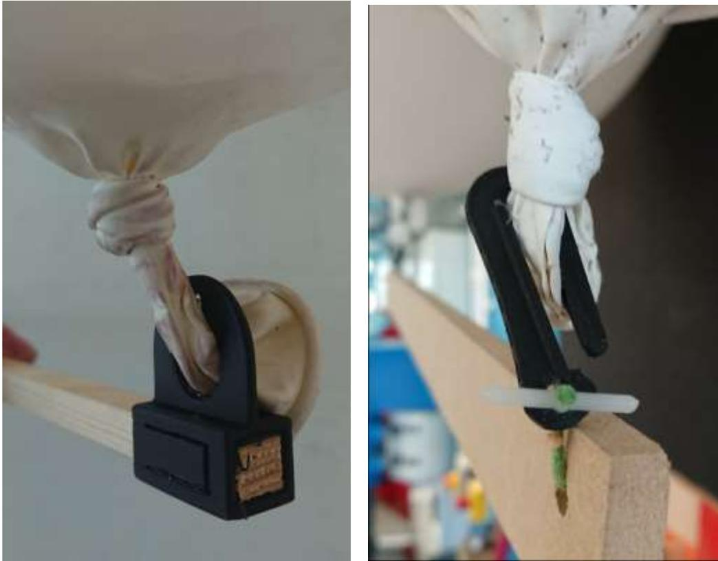
*Examples of 3D printed quick release balloon connectors from Cardinal Langley RC High School*
