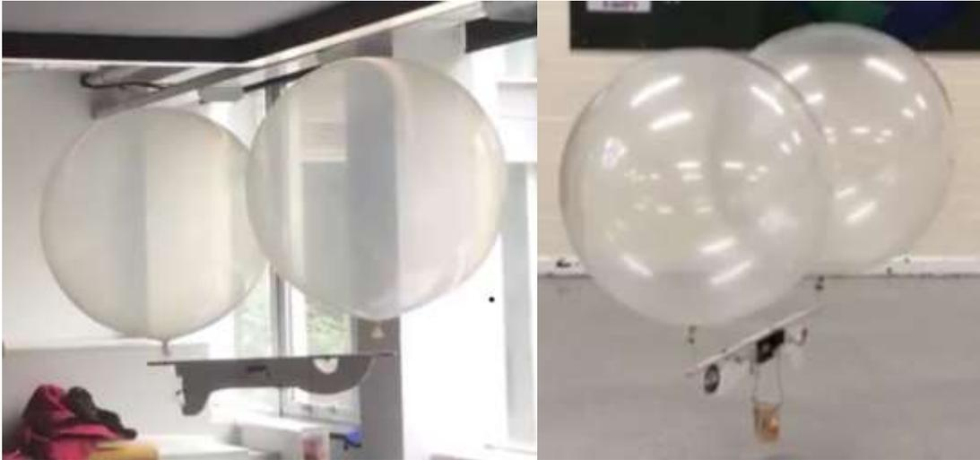
*Foamboard gondola suspended from a balsa spar. Three motors fixed in the X, Y and Z axes, control motion. No servos are used.*
