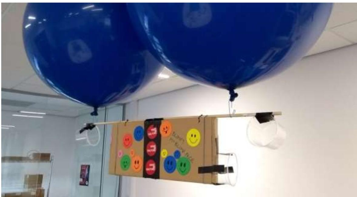
*This design uses 3 fixed nacelles to move the craft in the X, Y and Z axes.*
